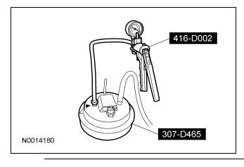
16. Allow the fluid to drain. Make sure that the fluid temperature is between 27°-49°C (80°-120°F). When the fluid comes out as a thin stream or drip, the fluid is at the correct level.
