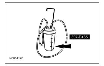
10. Hang the special tool under the vehicle. Position it upright and close to the transmission.
